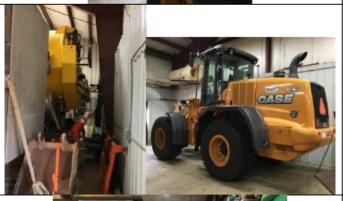
Vehicles are parked within an inch or two of walls and building structural columns with no bollard protection.
